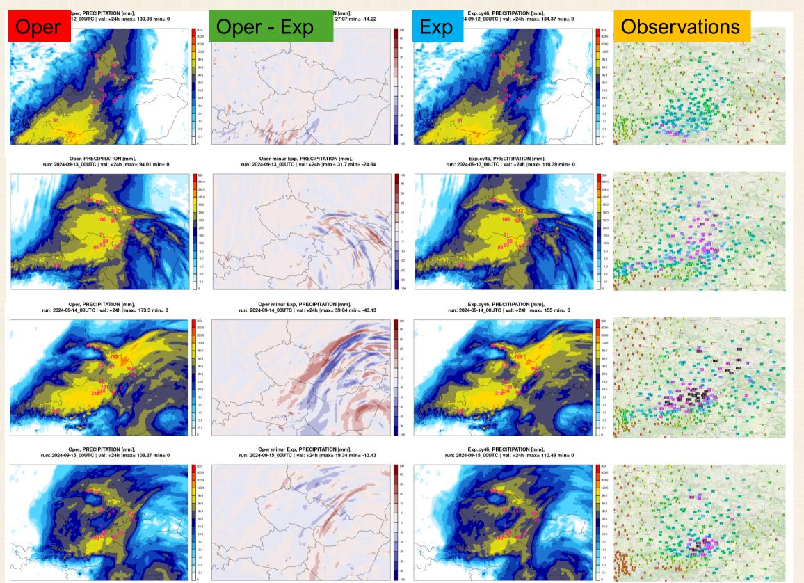
Comparison of prediction of cumulative precipitation (24h) : of operative model ALADIN/SHMU (Oper), experimental copy of Oper with Seviri and VarBC (Exp), difference the latest two setups and Observations.
